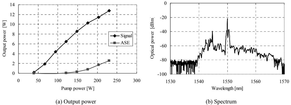
Figure 6. Amplification characteristics of the Er,Yb:glass waveguide with pulsed signal light
