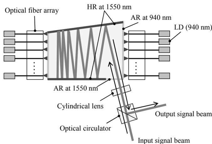
Figure 2. Optical path of the planar waveguide amplifier
