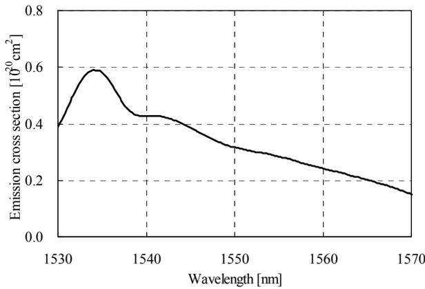
Figure 3. Emission cross section of Er,Yb:glass
