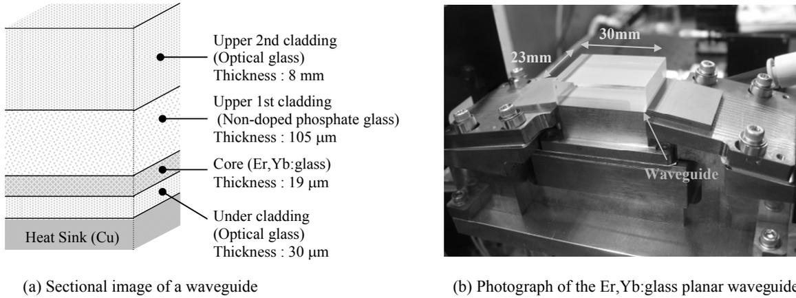
Figure 1. Structure of a double-clad Er,Yb:glass waveguide
