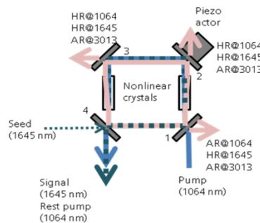
Fig. 4: View of OPO cavity for generation of the on-/off-line wavelengths.
