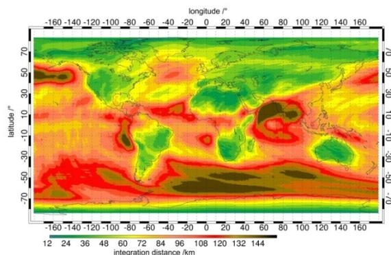
Fig. 6: Required along track integration distance in km (colour bar) required to achieve equal measurement precision of 1 % around the globe by MERLIN observations.
