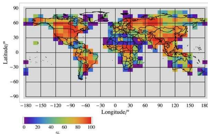
Fig 7: Relative error reduction (color bar) of monthly methane surface fluxes for July expressed by  $1 - \sigma_{\text{post}} / \sigma_{\text{pri}}$  where  $\sigma_{\text{pri}}$ ,  $\sigma_{\text{post}}$  correspond to the prior and posterior flux uncertainties, respectively. Credit: M. Heimann, MPI-BGC, Germany
