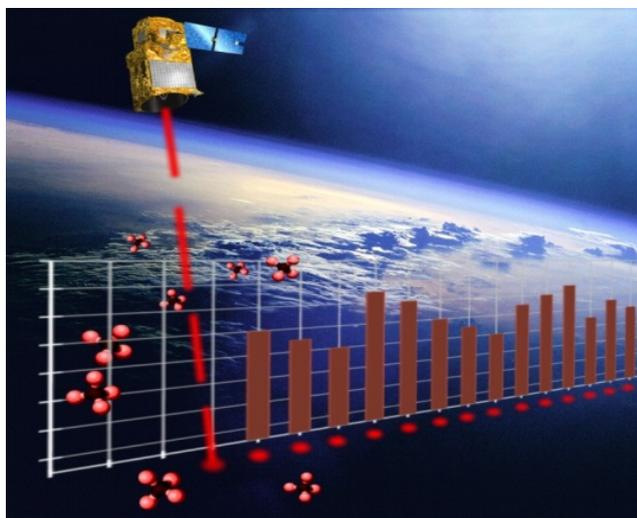
Fig. 1: Observational principle of the MERLIN instrument. Red bars symbolize the amount of  $\text{XCH}_4$  along the satellite ground track. Credit: CNES for satellite artist view, NASA for background photo
