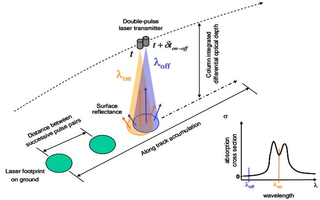
Fig. 2: Principle of IPDA lidar measurement using surface targets
